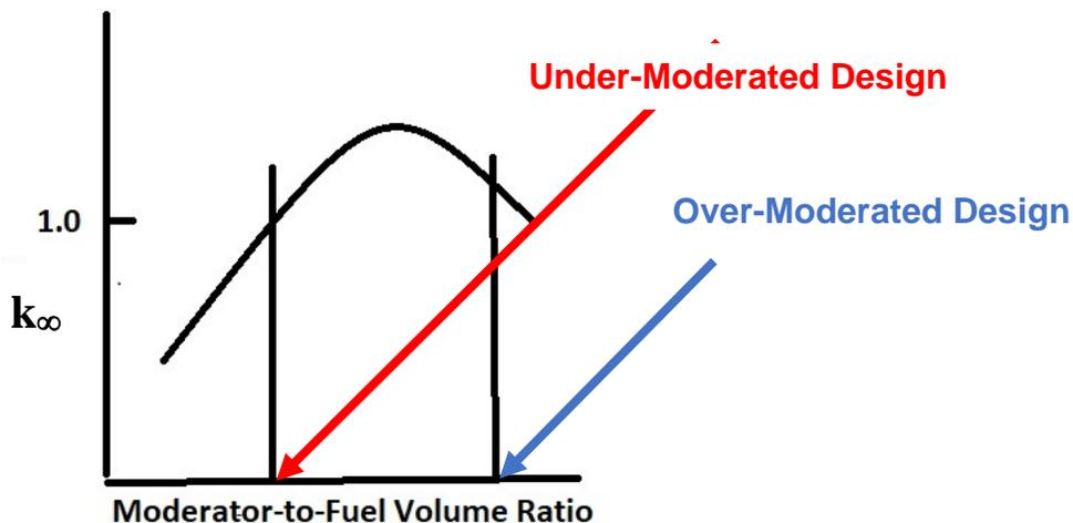
Figure 1. Moderator-to-Fuel Volume Ratio for Under-Moderation and Over-Moderation
