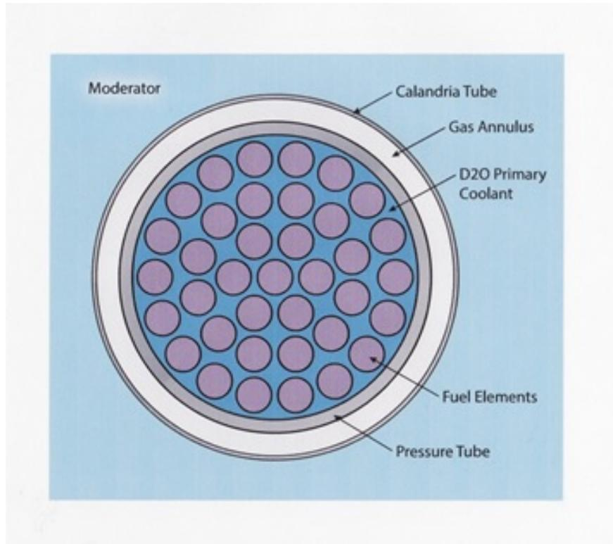
Figure 3. Face View of CANDU Basic Lattice Cell
