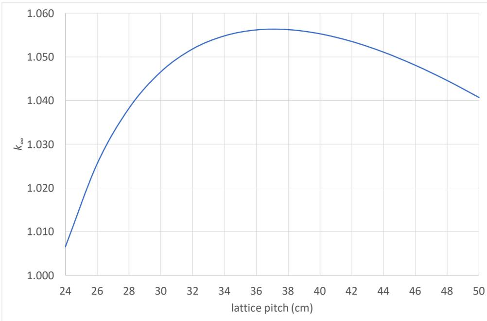
Figure 7.  $k_{\infty}$  as a Function of Lattice Pitch for an Equilibrium Core- DRAGON Result
