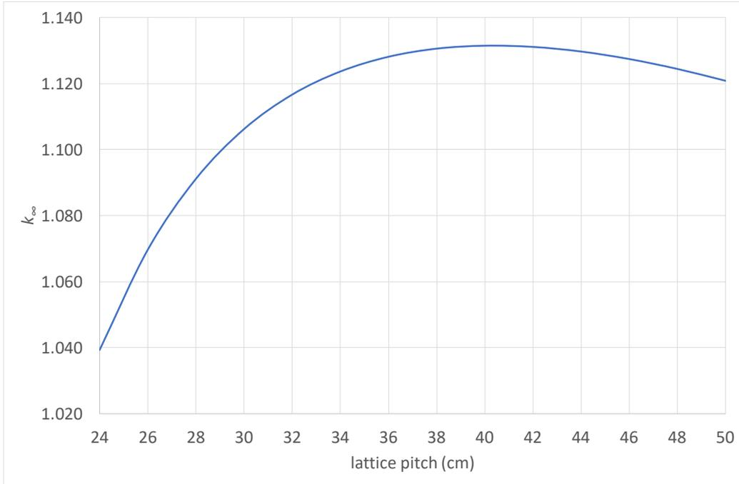
Figure 6.  $k_{\infty}$  as a Function of Lattice Pitch for a Fresh Core- DRAGON Result
