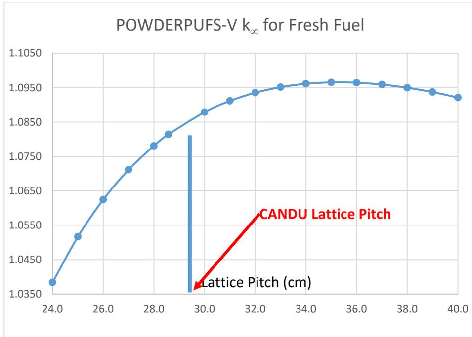
Figure 4.  $k_{\infty}$  as a Function of Lattice Pitch for Fresh Core - POWDERPUFS-V Result
