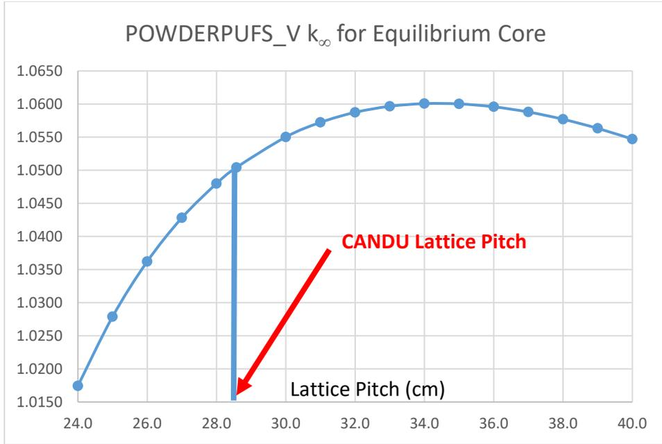
Figure 5.  $k_{\infty}$  as a Function of Lattice Pitch for Equilibrium Core - POWDERPUFS-V Result
